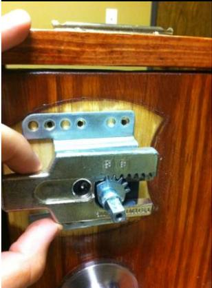
Take the security bar and the gear and proceed to place them on the lock. The backset should be adjusted to fit what type of door you're working on, whether it be 2 3/8 or 2 3/4. Most doors are going to fall under the 2 3/8 backset setting. **Note: Make certain that the teeth on the gear start right on the desired backset.** (An arrow is there for selecting desired backset)
