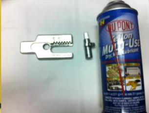
Grab your can of Teflon and apply some to the black part of the housing plate, the security bar, and the gear. This will ensure that the lock feels as fluid as possible when locking or unlocking the lock. **Note: Shake the can well before use**
