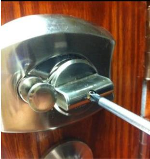
Insert the thumb knob on the door where the knob sits vertically when the lock is unlocked and horizontally when the lock is locked. The Ultimate lock logo should always read normally and not upside down when in the locked position. The screw that holds the lock can be installed as tight as your heart desires.
